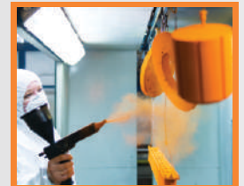
POWDER COATING UNIT
